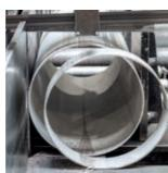
The plant in Niederaula is able to saw pipes of different diameters.
